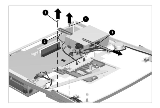
Figure 7-40. Removing the Docking Lever Cover
